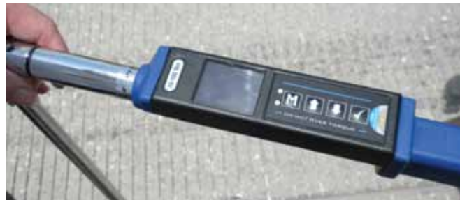
An electronic wrench that automatically sets the torque for airfield electricians is expected to decrease downtime for maintenance.
